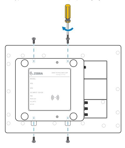
**3.** Use a 1.5 mm hex driver and turn clockwise to attach and tighten the four screws.
