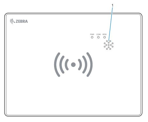
Lightly dampen a soft cloth and gently wipe the reader. Allow to dry before use.
